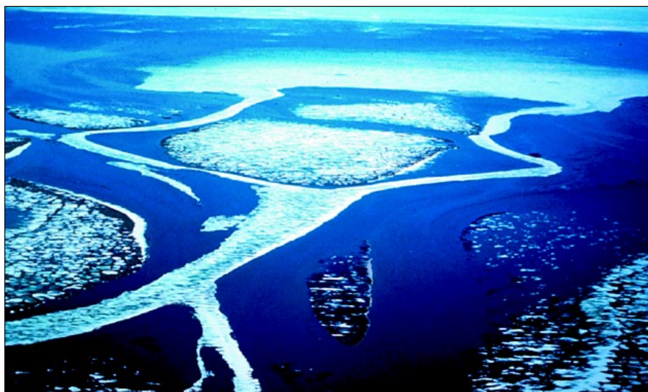
Floodwaters at the mouth of the Colville River delta in 1971. The LSU research team calculated that 10 days of flooding during breakup that year contributed 4.64 \times 10^9 \text{ m}^3 of freshwater—nearly half of that year's total discharge—as a freshwater wedge beneath 3,000 km 2 of sea ice (photo by Donald Nemeth).
