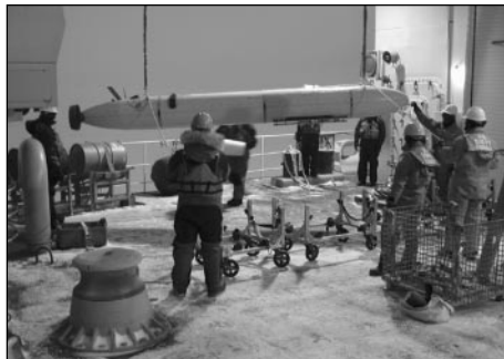
In late 2001, Healy supported testing of a new autonomous underwater vehicle (AUV) being developed at the Monterey Bay Aquarium Research Institute for the Atlantic Layer Tracking Experiment to help scientists determine what happens to Atlantic water as it enters the Arctic Ocean (photo by T. Walsh © MBARI 2001).
