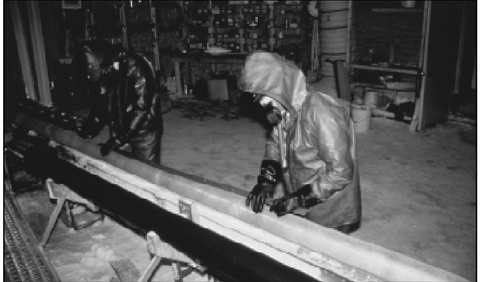
GISP2 investigators logging a freshly drilled 6-m ice core in the drill dome (photo by Mark Twickler).
