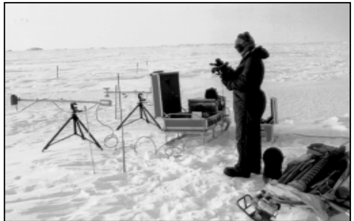
CRREL researcher measures the albedo of the sea-ice cover off Barrow, Alaska during the Office of Naval Research Electromagnetic Properties of Sea Ice (EMPOSI) field program. The objective is to monitor spatial and temporal variability in the reflected, absorbed and transmitted light as a function of ice conditions including ice that is snow-covered, bare, sediment-laden, bio-laden, melting and/or ponded.
