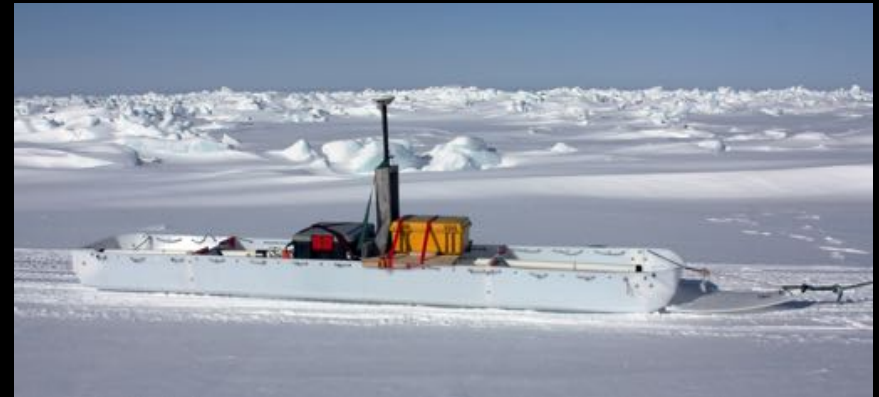
EM-31 (with DGPS) in sled for measuring ice thickness
