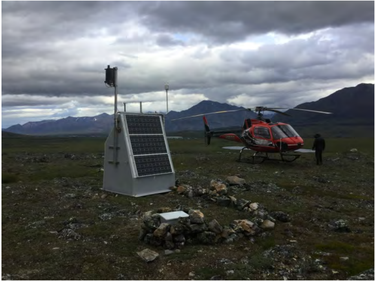
Photo of TA station E22K, located near Anaktuvuk Pass in the Brooks Range, on 18 July 2018. On this service trip, IRIS staff installed two additional lithium batteries and a wind turbine for extra power (the black cylinder on the left). The box in the foreground marks the top of the seismometer borehole. Photo by Max Enders, IRIS
